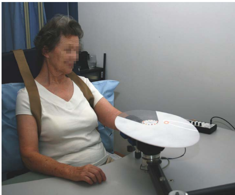
Figure 25: Stroke participant performing a tracking task using the robot showing the method of restraining trunk flexion
