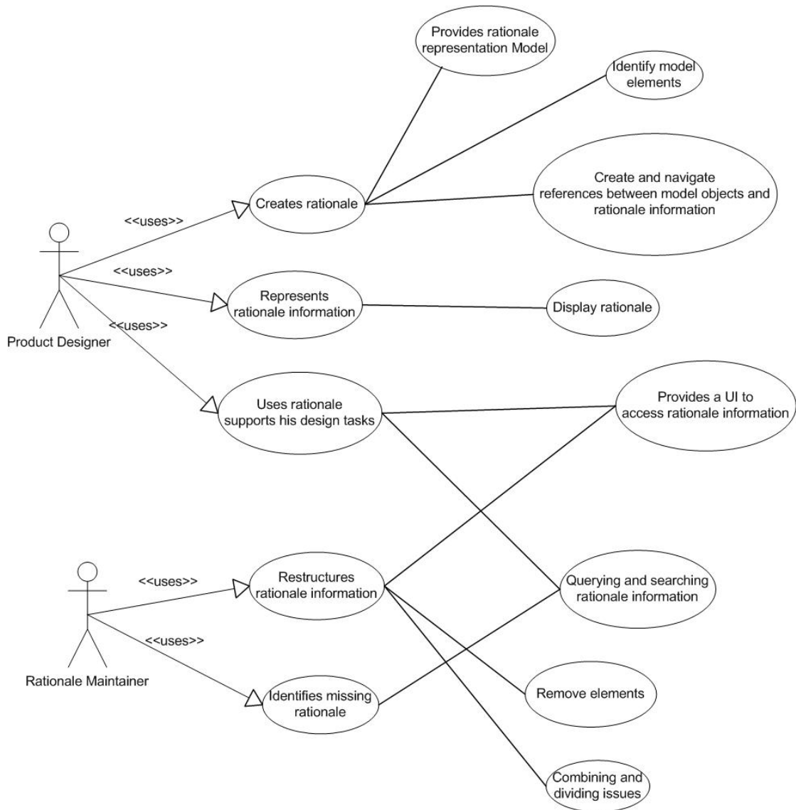
FIGURE 4.3: The use case for design rationale system identifying two users, the product designer and the maintainer of the rationale.
