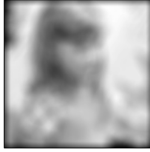
Figure 3.10: The result of performing a linear filtering operation the section of the image of ‘girl’ presented in Figure 3.7(a) using a flat, circular kernel of radius 10.
