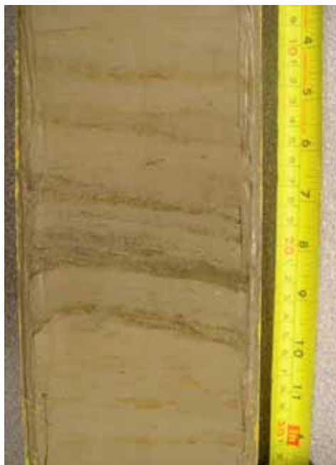
Fig. 6.8. A stacked sequence of thin silty turbidites, typical of the pre-6.4 ka interval in the canyon cores. Taken from core CD56837 in Cascais Canyon. Scale is in cm on the left and in inches on the right.
