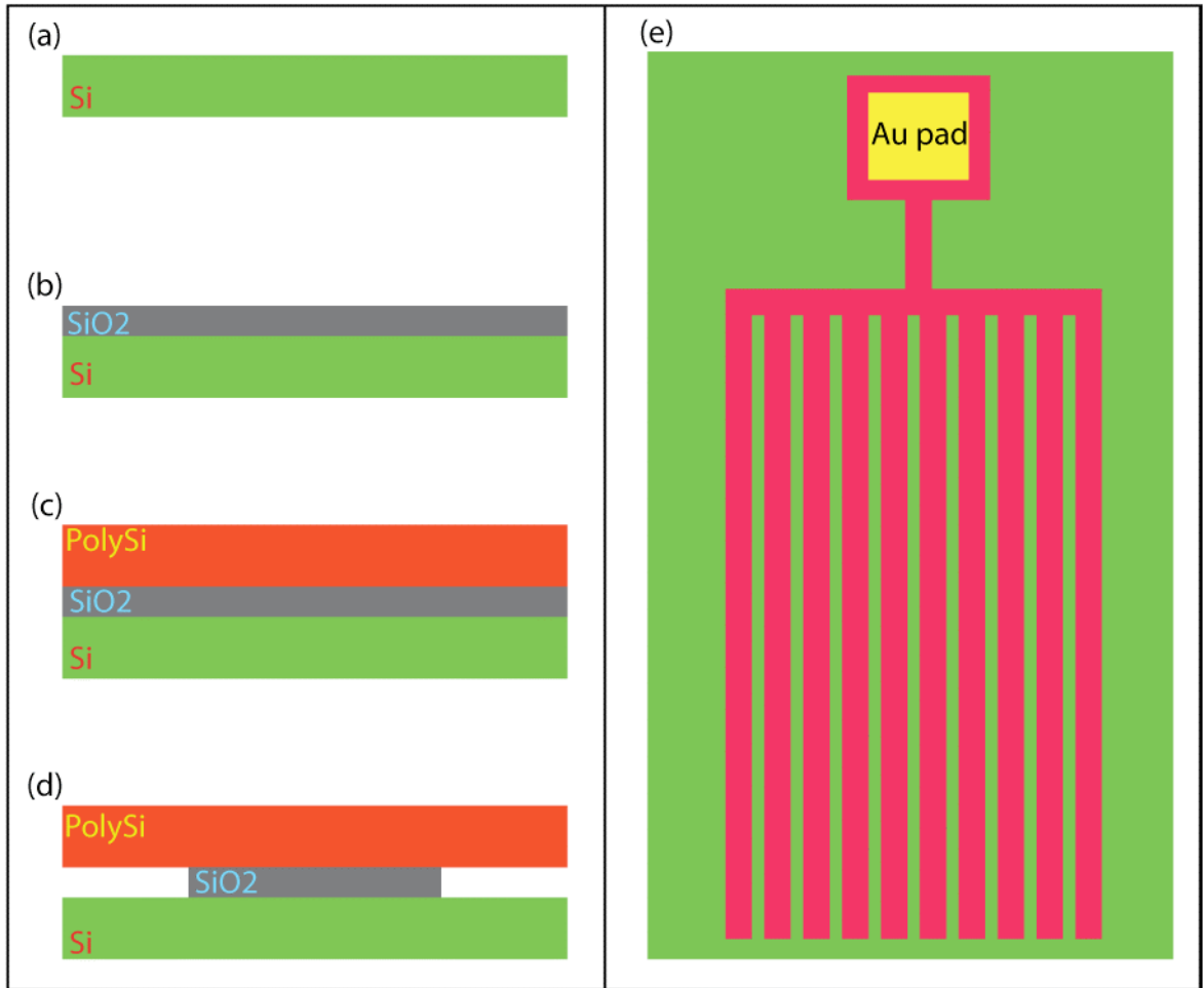
Figure 6-2 Fabrication process steps. (a) PSG was annealed on top of n-type Silicon wafer, then removed with HF. (b) \text{SiO}_2 was thermally grown on the silicon layer. (c) Polysilicon was deposited by LPCVD. (d) Polysilicon was defined with standard photolithography and patterned with reactive ion etching (RIE). (d) The oxide layer was undercut by wet etching with HF. (e) top view of the Polysilicon electrode structure. Gold was evaporated and patterned onto the contact pad to reduce contact resistance.
