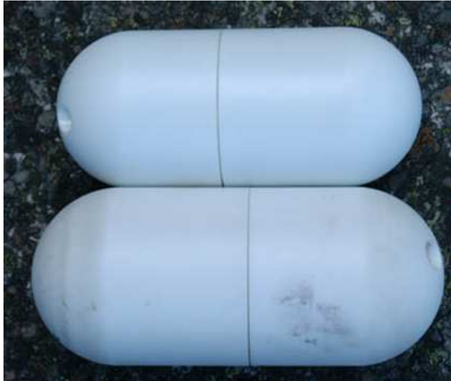
FIGURE 3.11: Size difference: The new smaller probes fit down the holes easier
