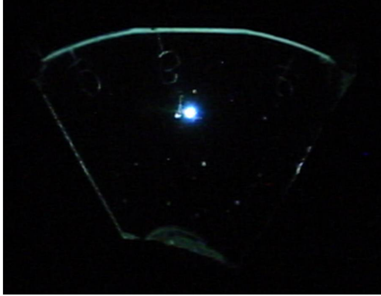
FIGURE 8.5: Photograph of the polariton laser operating above threshold.
