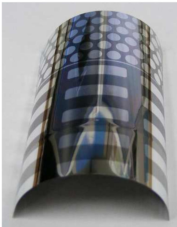
FIGURE 6.12: 1\text{cm}^2 nip substrate cells deposited on a molybdenum/Kapton flexible substrate. The 6\text{cm}^2 cells can be seen in the centre of the substrate, with more 10\text{mm}^2 cells defined behind them. The curvature of the substrate is due to thermal stress as a result of the mismatch between a-Si:H deposited at 200\text{C} and molybdenum at room temperature
