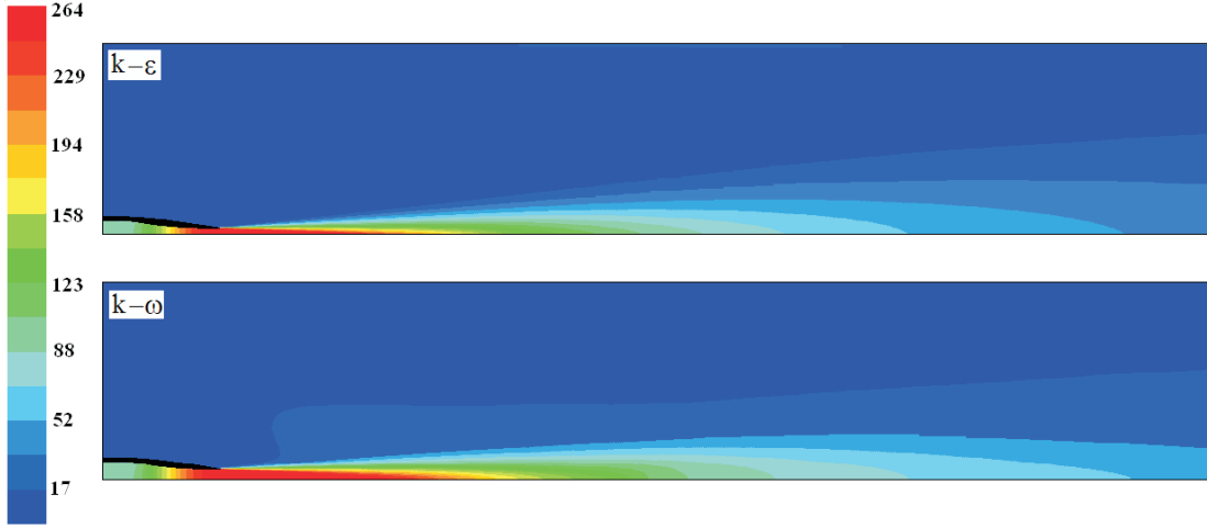
FIGURE A.4: Near-field comparison of k - \varepsilon and k - \omega models
