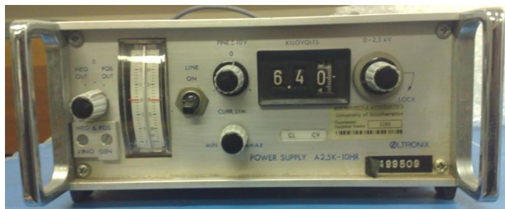
Figure 27: Secondary capacitor power supply, model Oltronix A2,5K10-HR.
