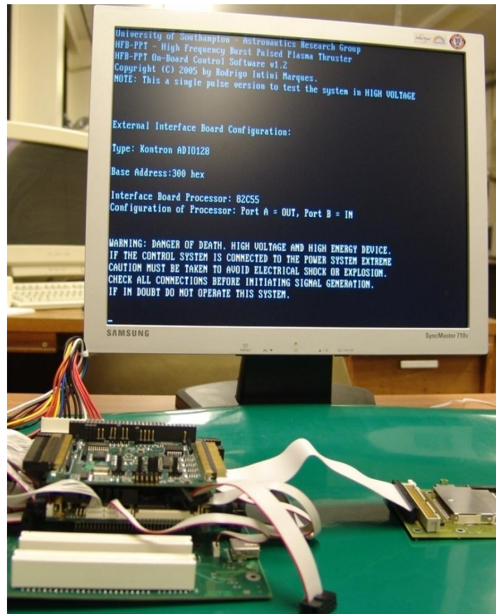
Figure 35: The software written in “C” language running on the PC-104 control system.
