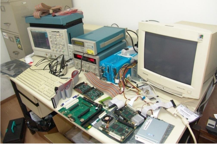
Figure 34: The calibration workbench for the PC104 Control System.
