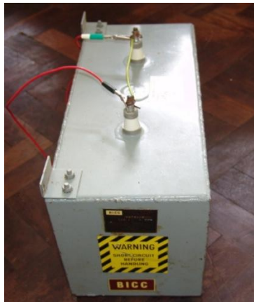
Figure 37: TS-PPT Main capacitor.
