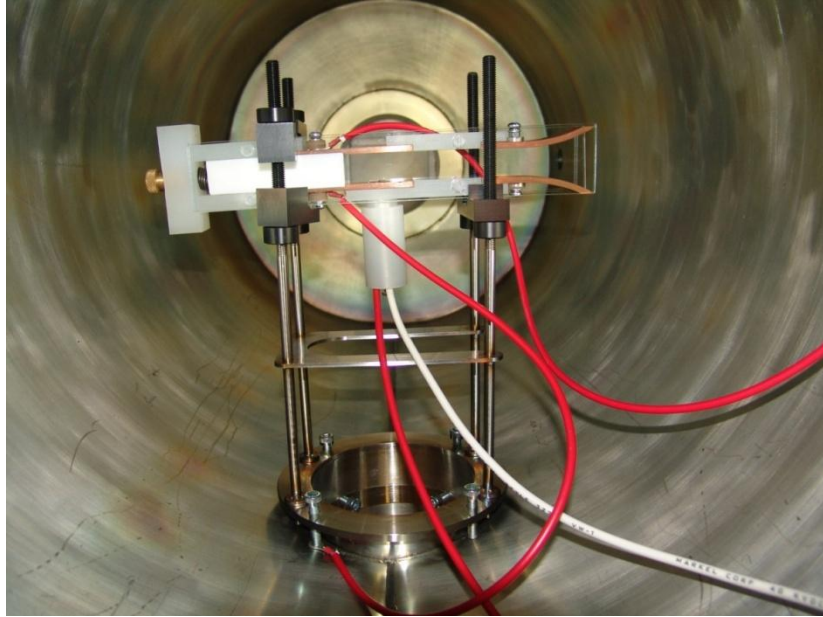
Figure 42: TS-PPT inside the vacuum chamber being prepared to be tested.
