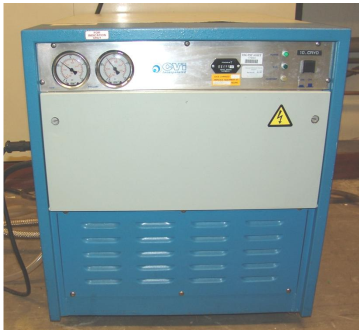
Figure 24: The cryogenic pump compressor.
