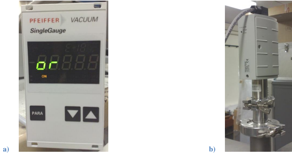
Figure 25: The Gauge controller (a) and the pressure gauge (b) installed on the facility.
