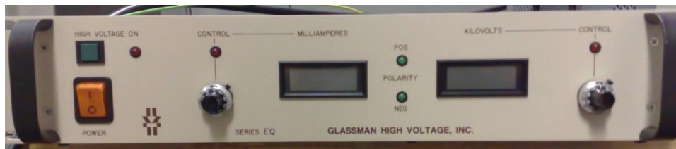
Figure 26: Primary capacitor power supply, model Glassman EQ10R120-22.
