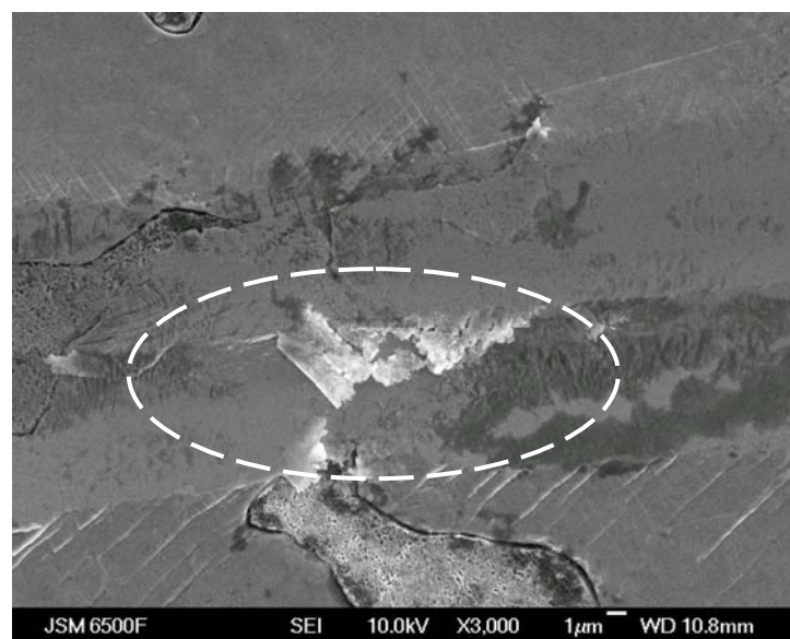
Figure 8.10: Multiple scratches made in 25% BS. Material detachment was found when new scratches ploughed along the edge of the previous scratches.
