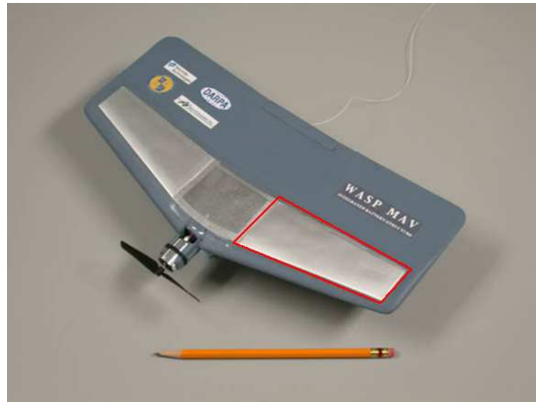
Figure 2-10 - AeroVironment Wasp showing multifunctional batteries on wings Battery on left wing outlined in red. (Image © 2002 DARPA.)
