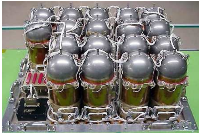
Figure 2-5 - Nickel-hydrogen battery (Image © & courtesy of JAXA)
