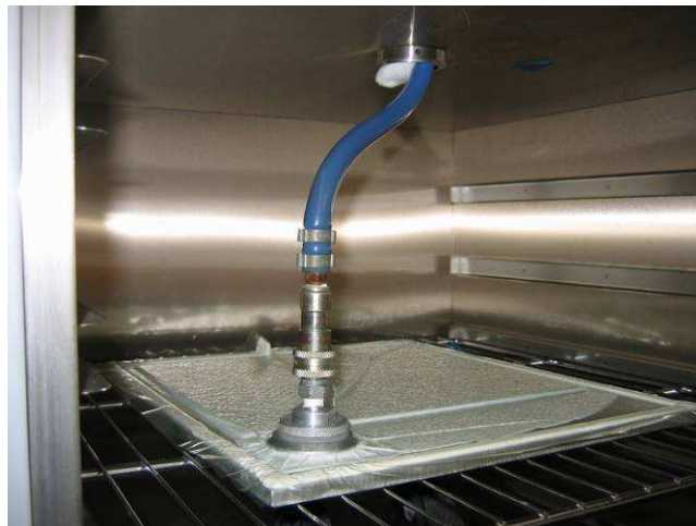
Appendix Figure E - The plate in the curing oven under vacuum
