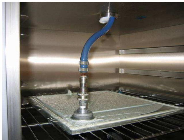
Figure 5-4 - The plate in the curing oven under vacuum
