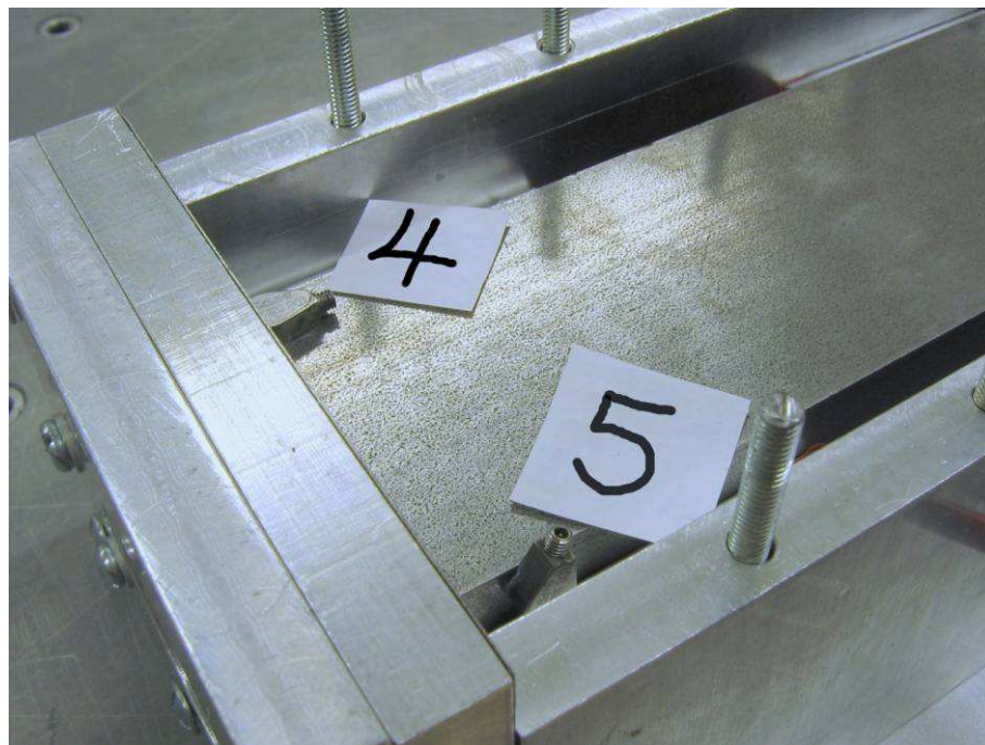
Figure 4-22 - Detail showing position of accelerometer channels 4 (vertical) and 5 (lateral)
