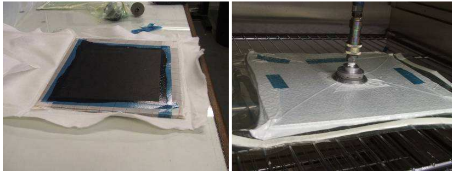
Figure 5-5 - Panel with peel ply (L) and vacuum bagged in the oven (R)
