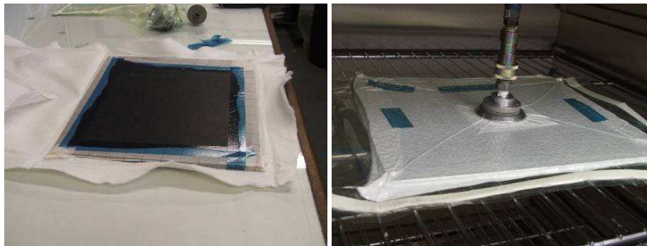
Appendix Figure G - Panel with peel ply (L) and vacuum bagged in the oven (R)
