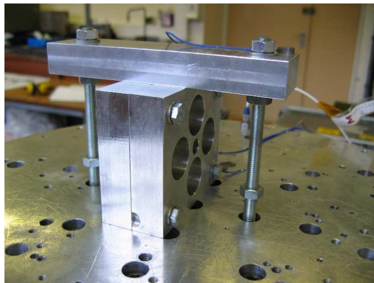
Figure 4-5 - The jig attached to the shaker
