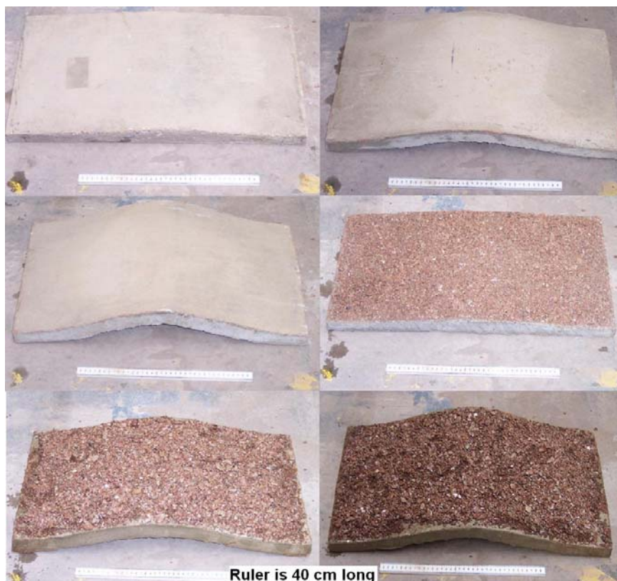
Plate 3.1 Concrete Antidune Bedform Inserts
