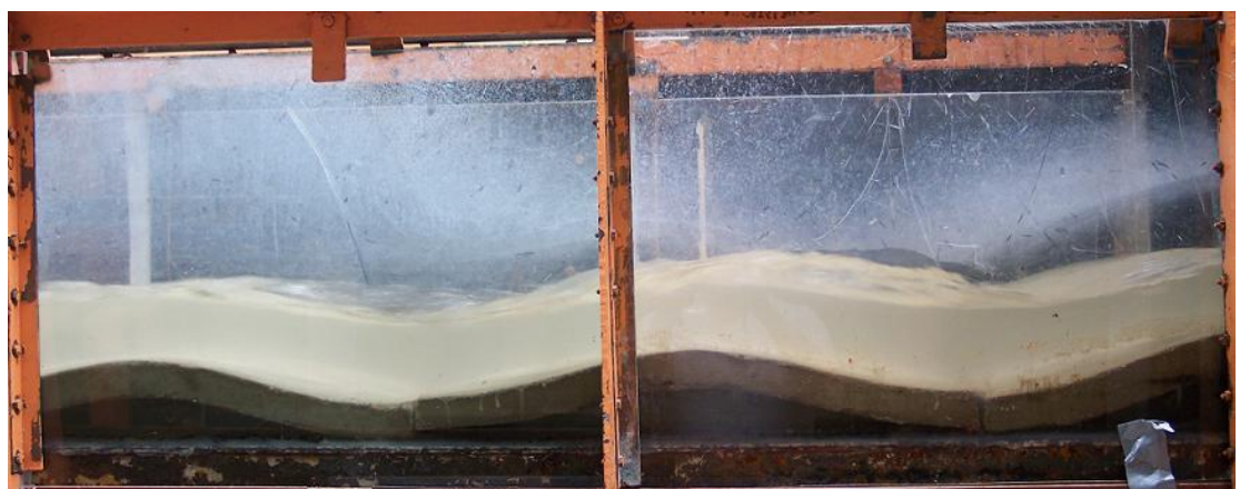
Plate 3.3 Concrete Inserts in-Flume
