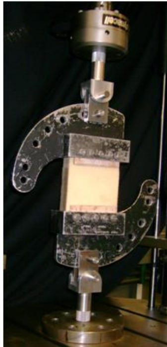
Figure 1 Modified Arcan rig
