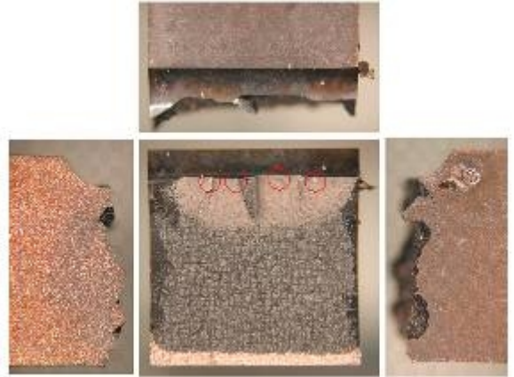
Figure 141 René N5 Bar 2 OB \Delta\varepsilon=1.38\% , 2573 cycles to failure
