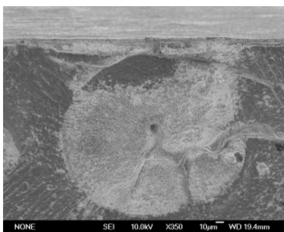
Figure 168 - SEI micrograph Subsurface initiation point Orientation A, 725°C
