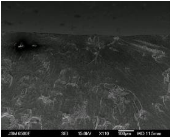
Figure 196 - SEI micrograph Initiation site A (Figure 195)
