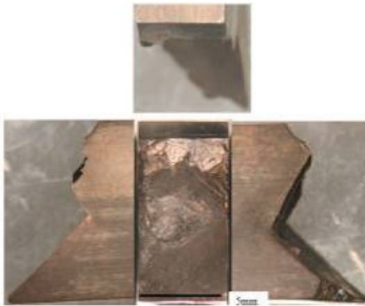
Figure 148 BAR P24-A, OB \Delta\epsilon=1.19\% , 127649 cycles to failure
