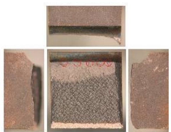
Figure 143 René N5 Bar 4 OA \Delta\varepsilon=1.38\% , 4945 cycles to failure
