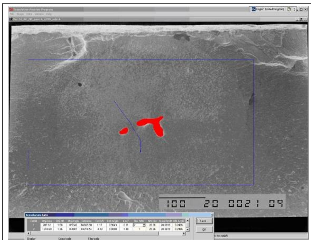
Figure 222 Pore area calculation using TAP software
