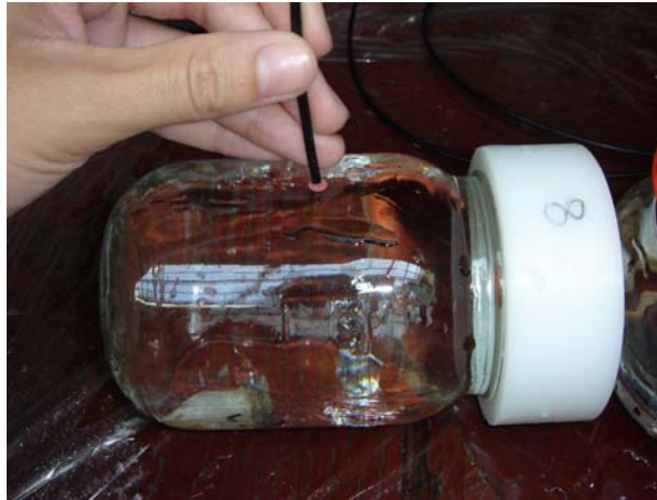
Figure 5.3 Taking a measurement from a respirometer in the Tropical Marine Science Institute aquarium, National University of Singapore. The end of the fibre optic cable is placed on the glass where the oxygen sensitive foil is glued on the inside.
