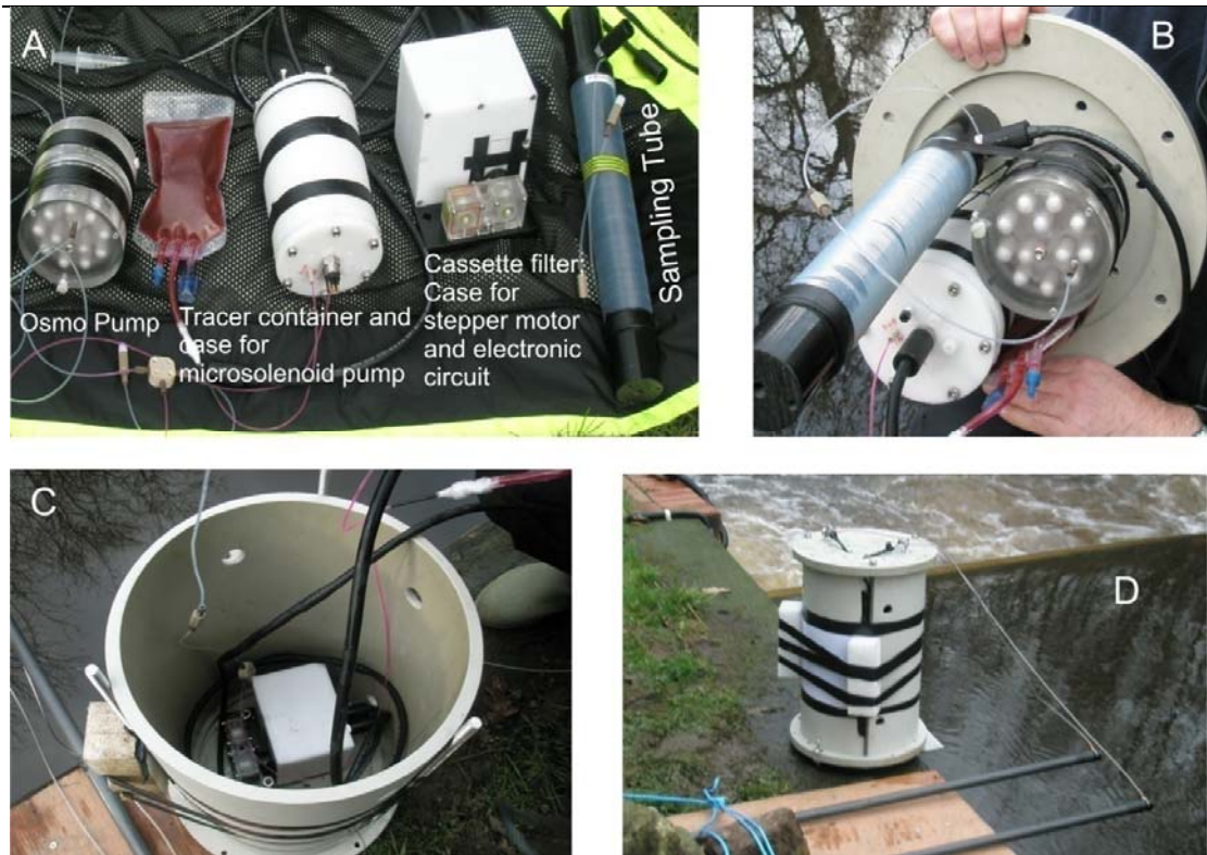
Figure 3-11: MK II prototype of SCAWS. A: Parts of SCAWS; B: Configuration of Cassette filter and electronics case; C: Configuration of osmo pump and tracer injection system; D: Complete SCAWS prior deployment.
