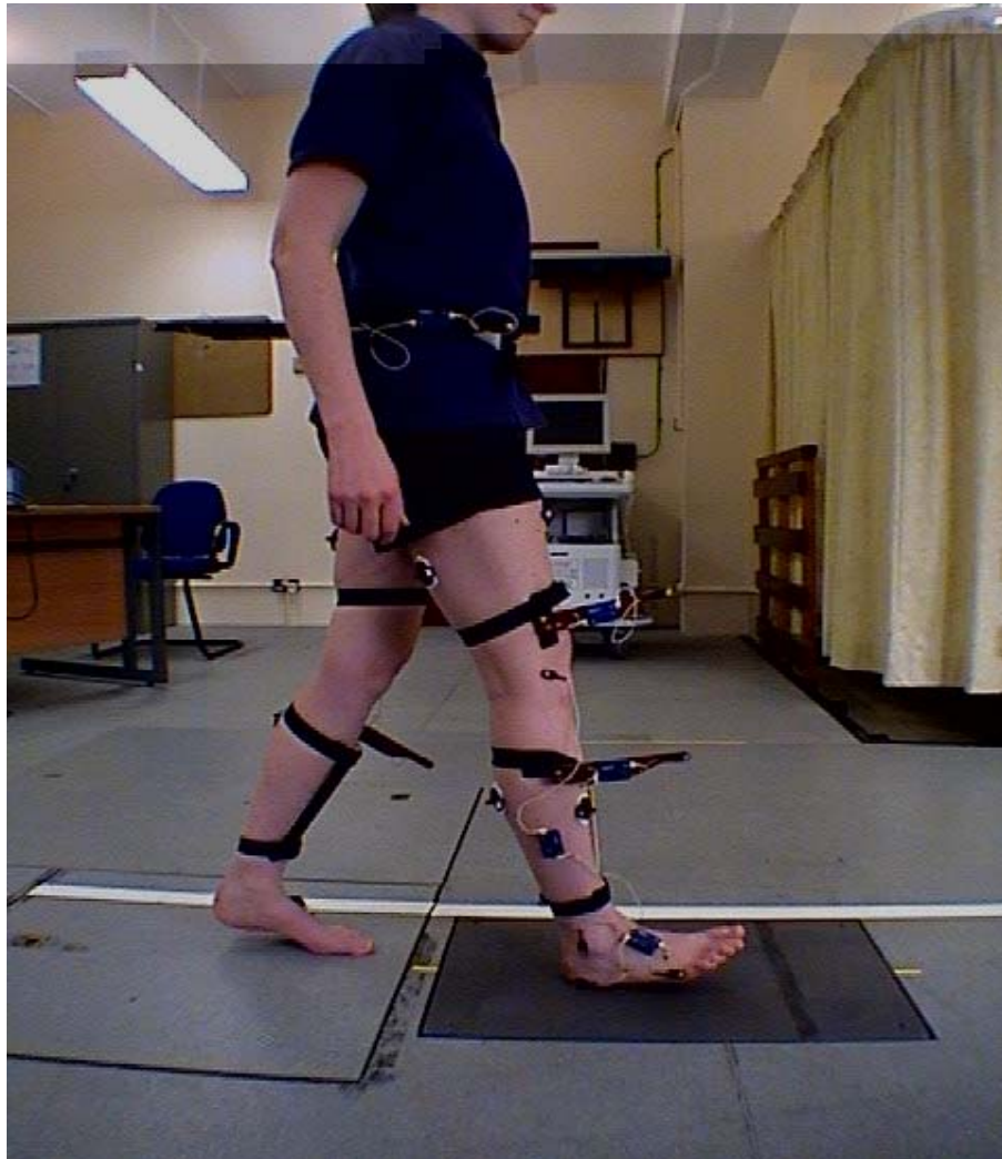
Fig 3.2.2 A gait analysis trial with subject walking with markers set up.
