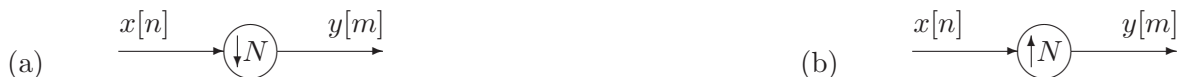
Fig. 3.4: Basic multirate operations for sampling rate alteration: (a) decimation; (b) expansion of signal x[n] by a factor of N .
