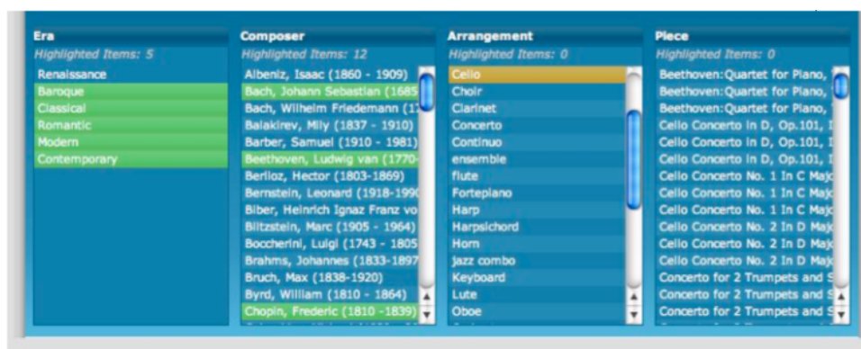
FIGURE 3.5: A prototype of Backward Highlighting was created on a set of mSpace columns and studied separately from the typical style of mSpace interface, shown in Figure 2.21. As mSpace columns filter left-to-right, Backward Highlighting highlights relationships backwards against the flow of filtering.
