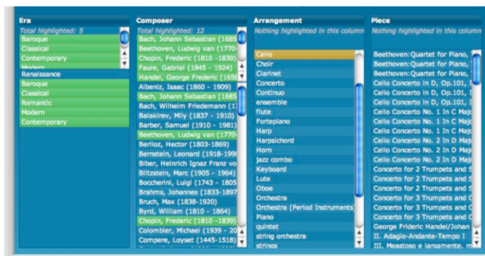
FIGURE 3.6: Bucket Highlighting, which copies highlighted items into a separate list at the top of each mSpace column, was prototyped in a similar stripped back interface and compared to Backward Highlighting.
