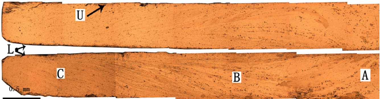
Fig. 4 Optical microstructure of a cross section of the Al-1Mg-4Cu disk subjected to HPT. L denotes lower surface and U denotes upper surface.
