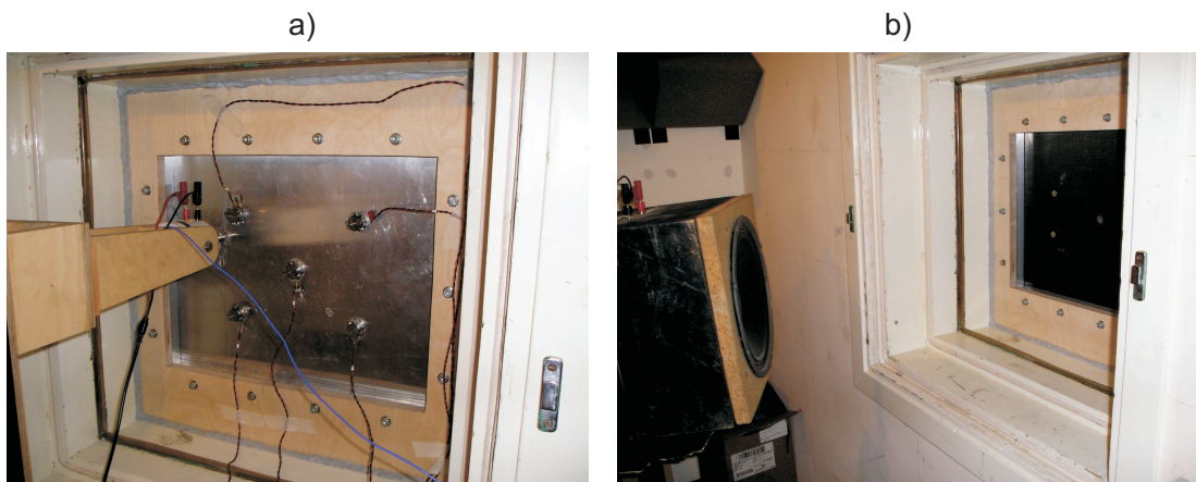
Figure 5.20: Set-ups for shaker excitation (a) and loudspeaker excitation (b).
