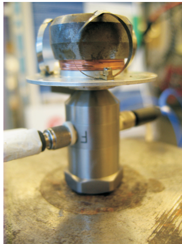
Figure 4.2: Set-up for blocked force measurement.
