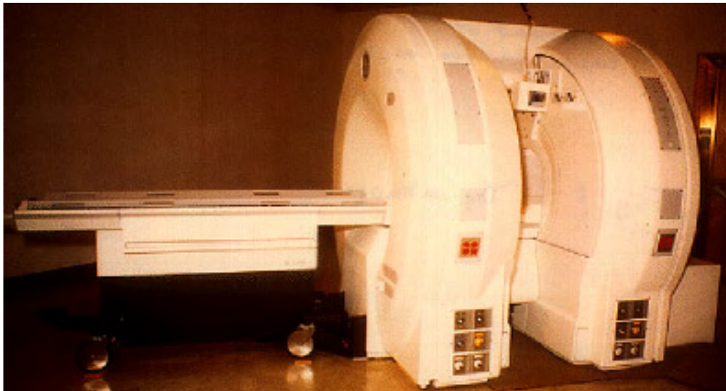
FIGURE 4.5: Image of split coil MRI note the size of the gap between the rings (image from Martin et al. (1998))
