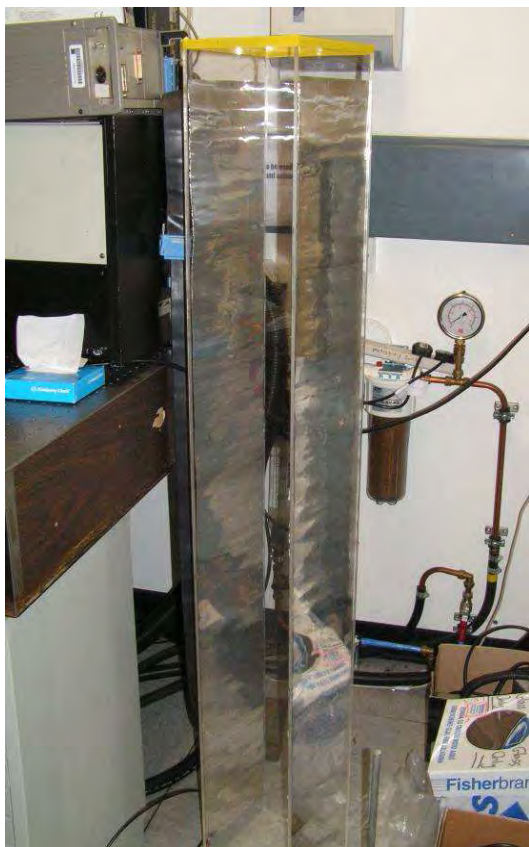
Figure 4.48 Static separation tower, comprising two parallel plates to produce an electrical field which could separate falling particles according to their charge.
