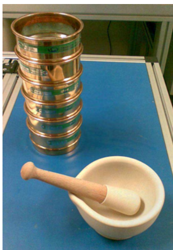
Figure 4.43 Metal sieves, pestle and mortar used for crushing and separating particles.
