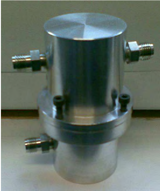
Figure 4.22 First dust blowing system, containing a mesh. It did not work because the velocity of gas was not high enough
