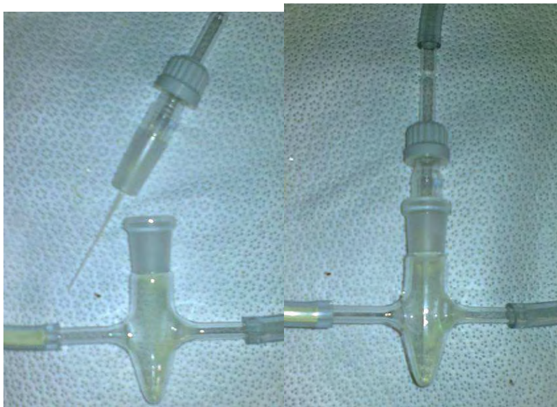
Figure 4.23 Dust blowing system consisting of a flask containing dust through which gas can flow and a nozzle to lift the dust
