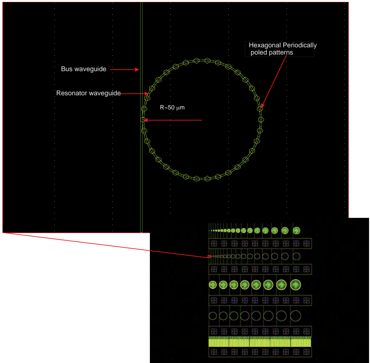
Figure 7.3: Pictures of the designed photomasks with the waveguides and the periodic hexagonal patterns
