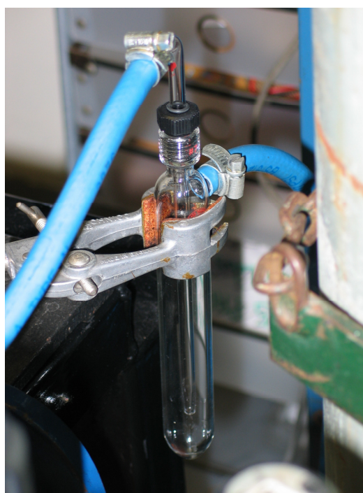
Figure 13.2. Device to Saturate with N 2 with H 2 O.
