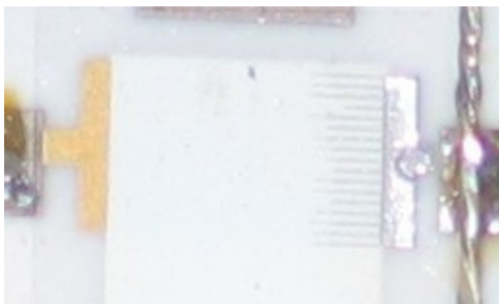
Figure 13.9. Damaged Type 1 Sensor (102) covered with Quartz window.
