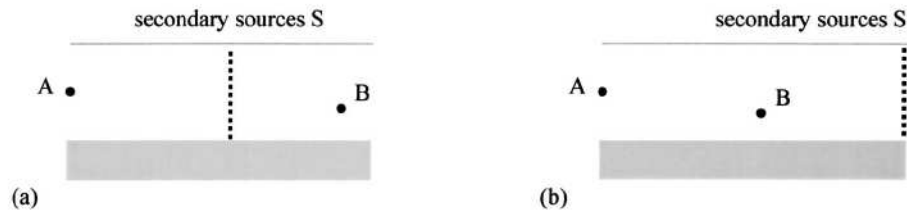
FIGURE 3.7: Problem definition for measuring the Green's function between points A and B using secondary sources S . From ref. [45].
