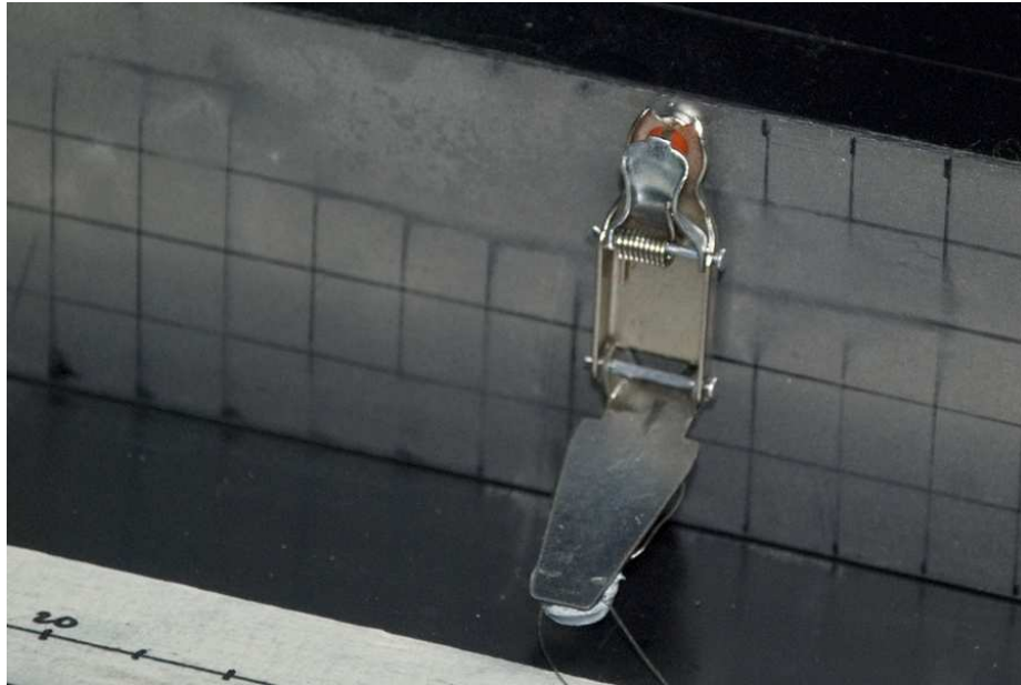
FIGURE B.1: Device used to trigger the pseudo-impulsive sources. The markings are at 10 mm intervals, and give an indication of the size of the setup.
