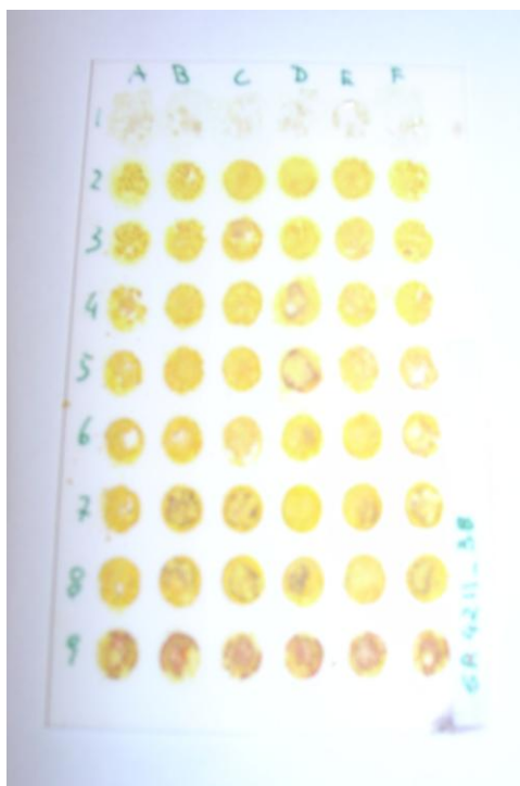
Figure 3.3 – BiMoVOX array, fired at 700°C in oxygen atmosphere, displaying the ring effect
