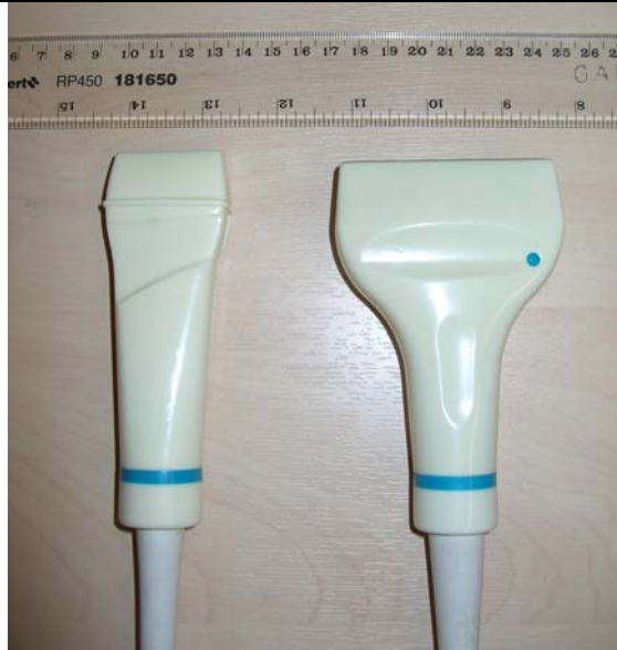
Figure 20. Photograph of the Diasus MSUS system 8 – 16MHz (active length 26mm) and 5 – 10 MHz (active length 40mm) transducers.
