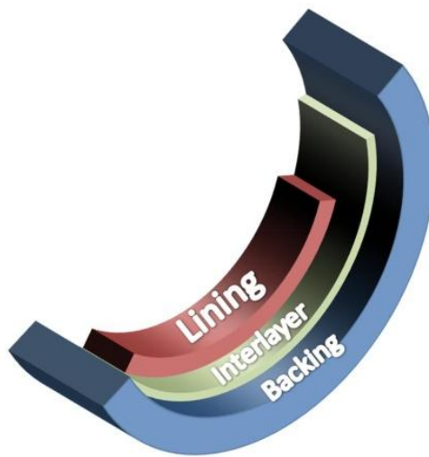
Figure 8. Tri-layer architecture displaying backing, interlayer and lining layers.
