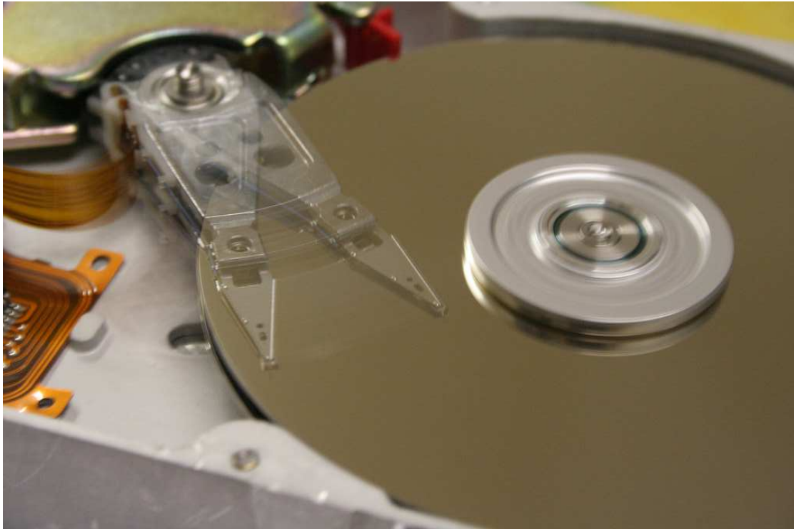
FIGURE 3.1: Image 4 of the inside of a hard disk (without cover) showing the read/write head moving across the spinning platters.
