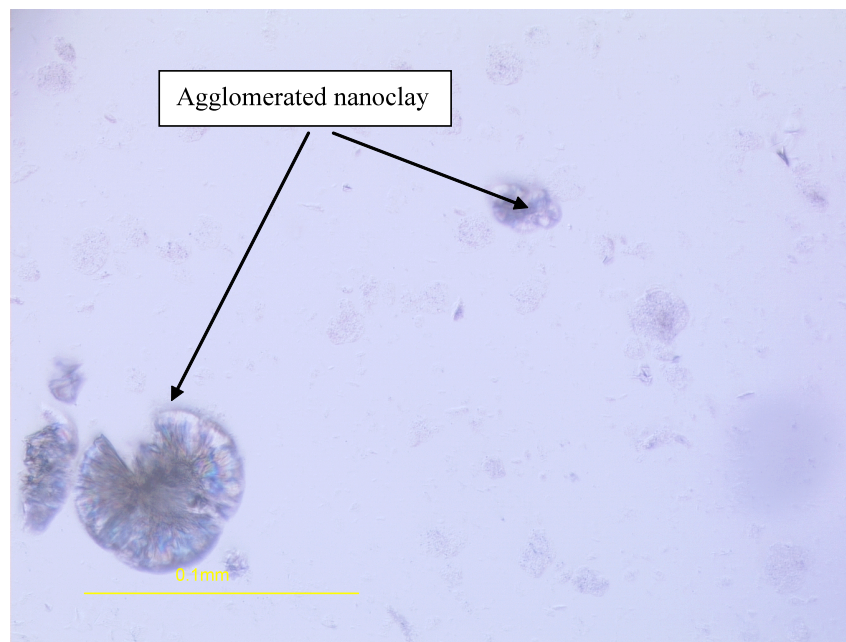
Figure 5-3. 3% I.30E 200x. showing expanded nanoclay agglomeration.
