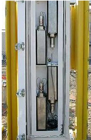
Figure 2.3: A typical NaI(Tl) based portal configuration showing 4x NaI(Tl) detectors in each of the portal's panels [Pacific Northwest National Laboratory, 2009].
