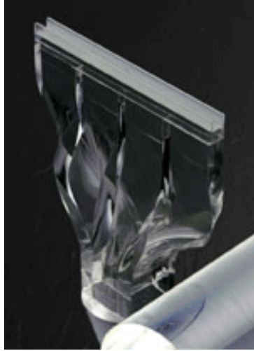
Figure 3.4: An example of a twisted light guide used for piping light from a thin sheet to a round surface [Saint Gobain, 2009a].
