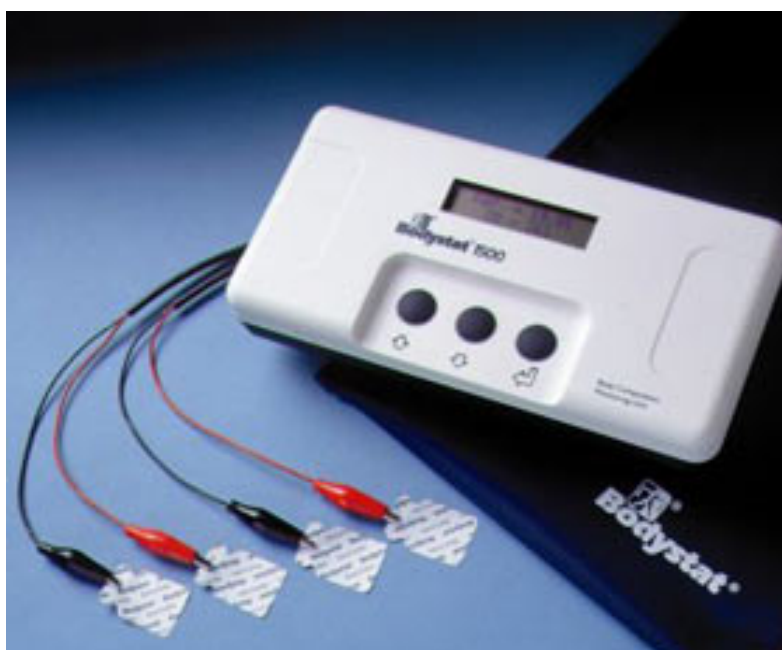
Figure 2.2 Bodystat® displaying the four electrodes that is used to measure fat and lean mass.
