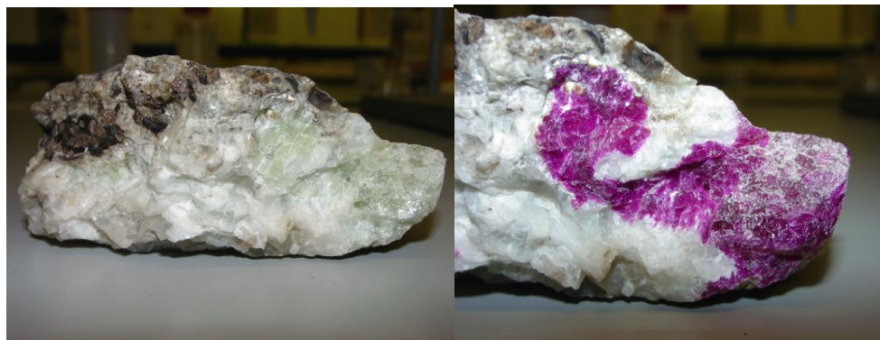
Fig 5.1 Photographs of a natural sample of hackmanite before and after exposure to UV radiation at 254nm
