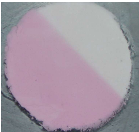
Fig 5.15 A photograph of a sodium chloride containing hackmanite partially exposed to 254 nm UV radiation showing a distinct colour change from white to pink
