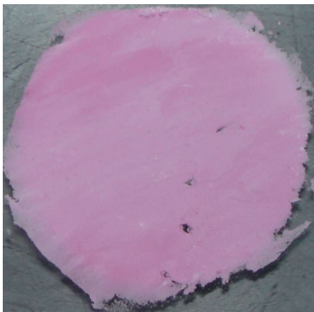
Fig 5.28 Photograph showing the colour of tenebrescence of a sodalite containing chloride and potassium replacing some sodium in the structure
