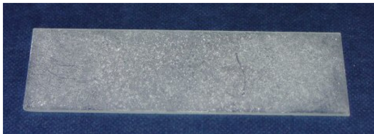
Fig 8.11 Photograph of a zeolite A film formed by self assembly using hexanoic acid on a glass microscope slide
