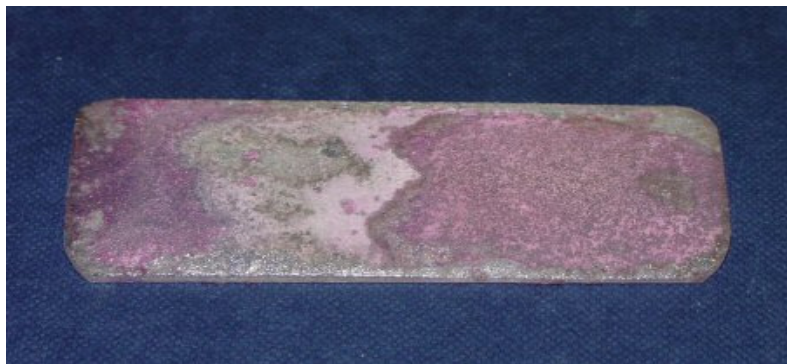
Fig 8.17 A photochromic sodalite film produced by thermal conversion of a zeolite A film under reducing conditions shown in the coloured state
