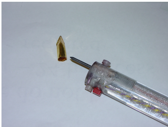
Fig 7.1 The welding tool and an example of a gold capsule before being welded shut
