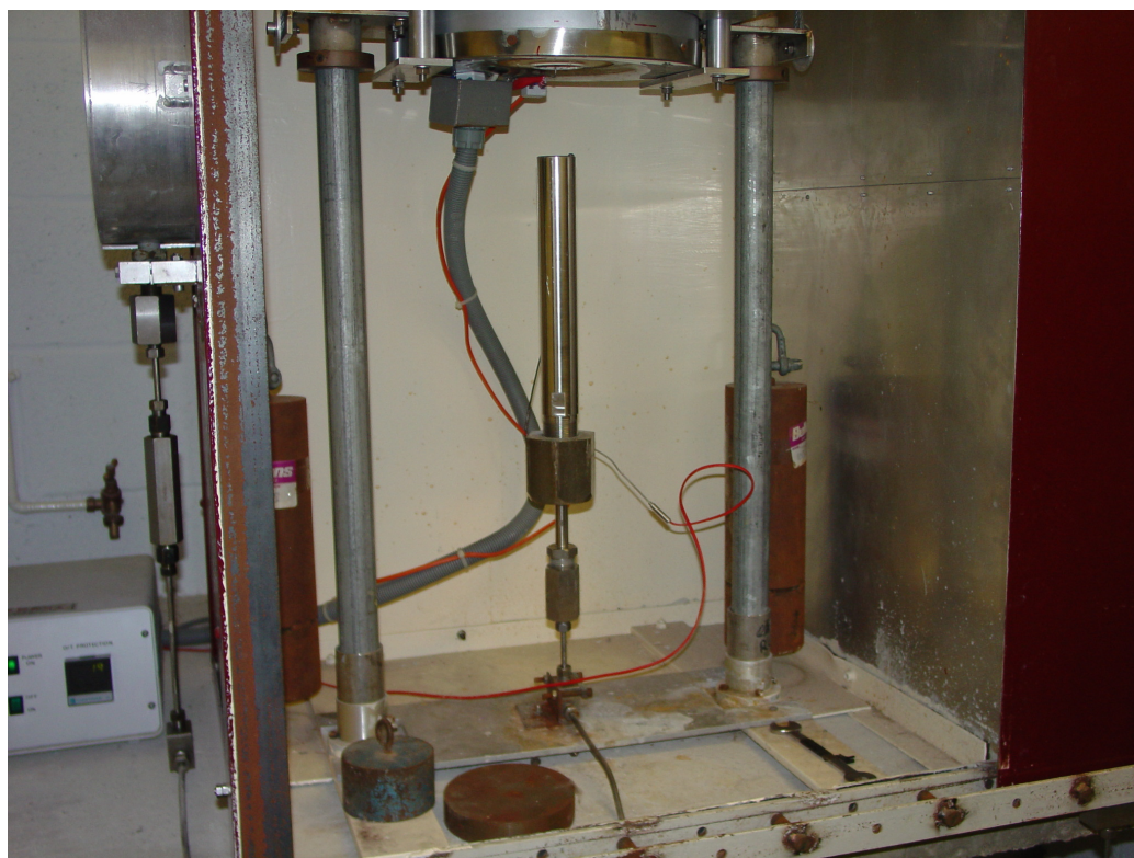
Fig. 7.2 Photograph of the hydrothermal rig showing the vertically mounted reaction vessel, reinforced furnace and steel safety cabinet
