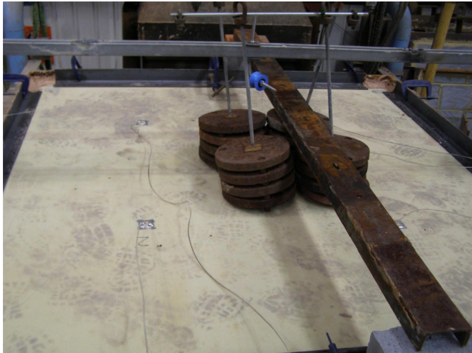
Figure 7.3: Unexposed face of the panel with loading weights in place before the fire was started
