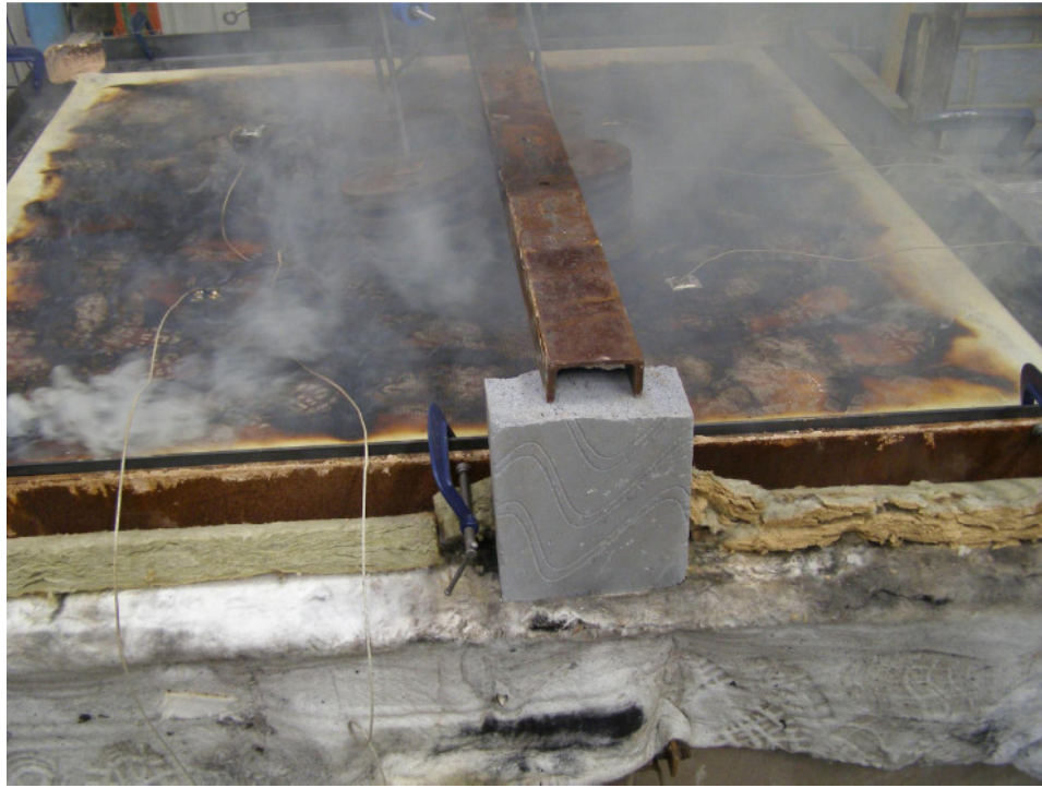
Figure 7.5: Unexposed face of panel after approx. 39 minutes showing darkening of surface and dense smoke
