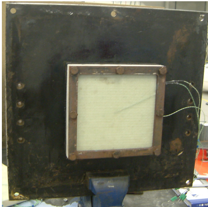
Figure 4.4: Clamping arrangement for test samples
