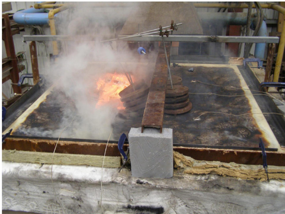
Figure 7.6: Unexposed face of panel after approx. 51 minutes showing flames protruding through hole
