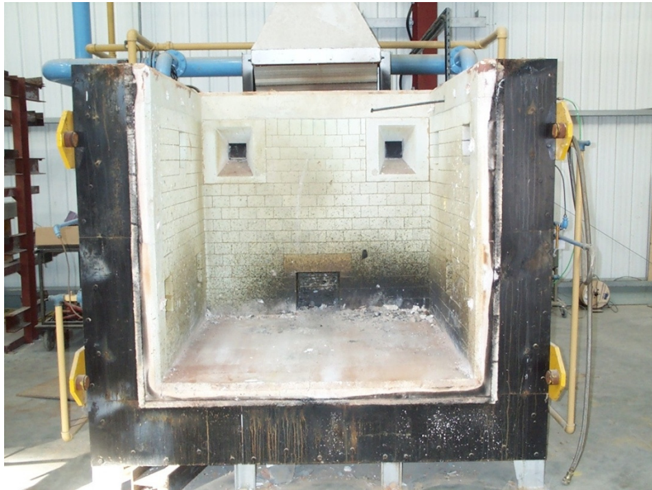
Figure 7.1: 1.5\text{m} \times 1.5\text{m} fire resistance furnace
