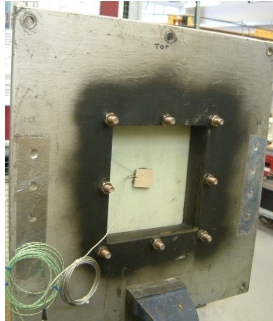
Figure 4.2: Detachable front plate holding test sample
