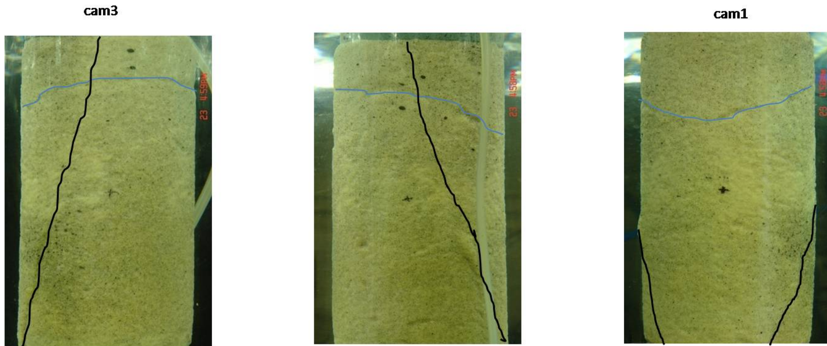
FIGURE 5.20: Photographs of the sample tested at 25 kPa taken at the end of the test. The sketches show the positions of shear bands.
