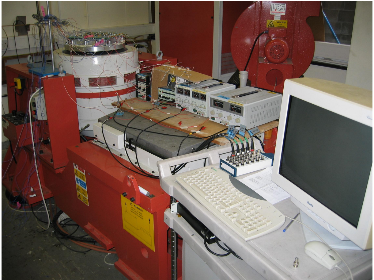
Figure 7.4: Entire experimental set-up (from left to right) shaker head with fully supported PCB attached, power supplies and detector circuits, continuity testing computer. Not shown: shaker control computer and dynamic signal acquisition computer.
