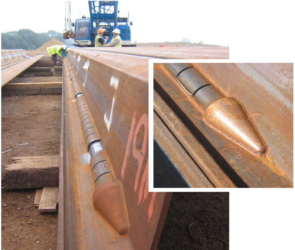
Figure 7-3: Instrumented section of the pile showing the cover plates and pointed tip (Structural statics, 2008)
