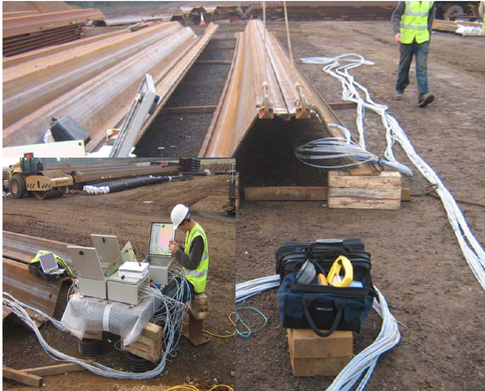
Figure 7-8: Self bending test to calibrate and check the strain gauges and temperature sensors
