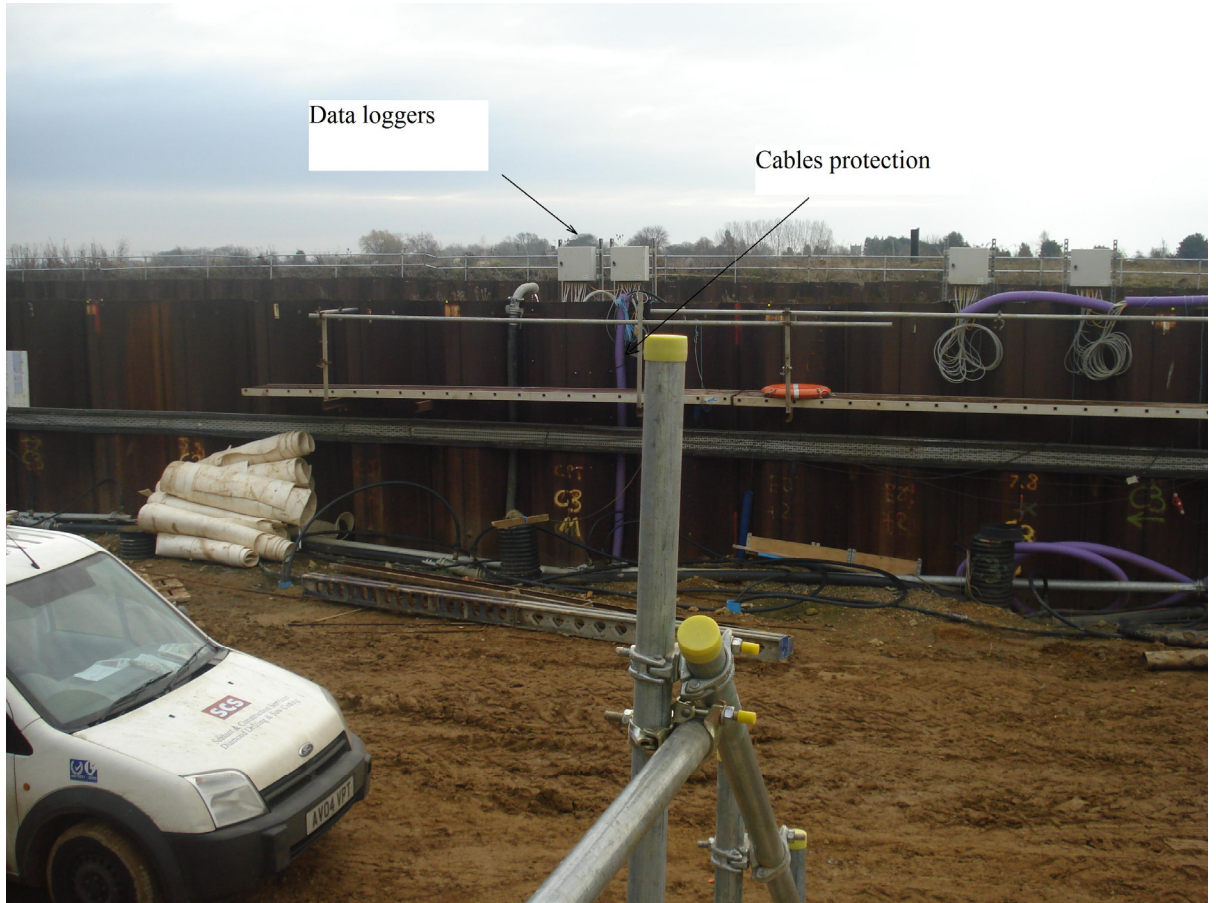
Figure 7-14: Data loggers installed on cell C3
