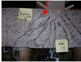
Figure 3.13 Crack distribution on B4A4 front surface at failure step
