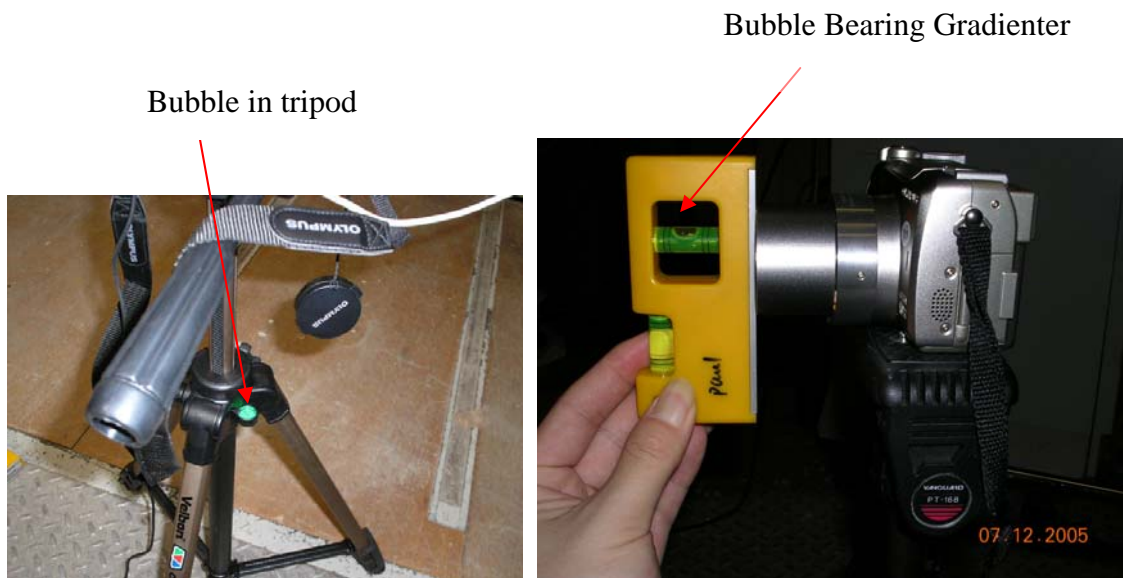
Figure 4.4 Tripod kept horizontal and camera (lens) kept vertical
