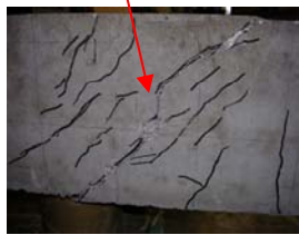
Figure 3.14 Crack distribution on B4A2 back surface at failure step
