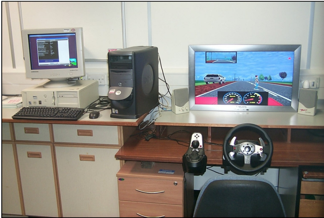
Figure 4.1 The STISIM driving simulator. The systems monitor to control the simulation is on the left.
