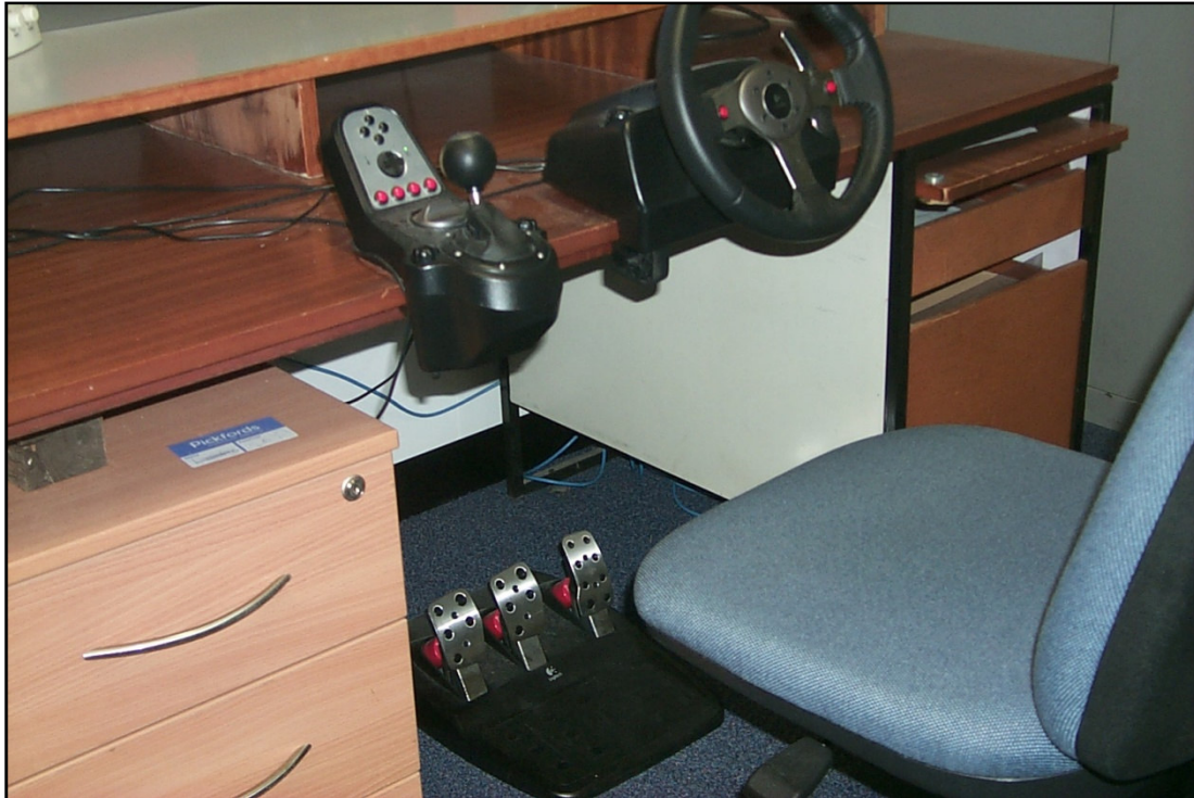
Figure 4.2 The STISIM driving simulator with the pedal assembly and the steering wheel in view.
