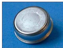
Figure 17: DS1921 I-button temperature datalogger
