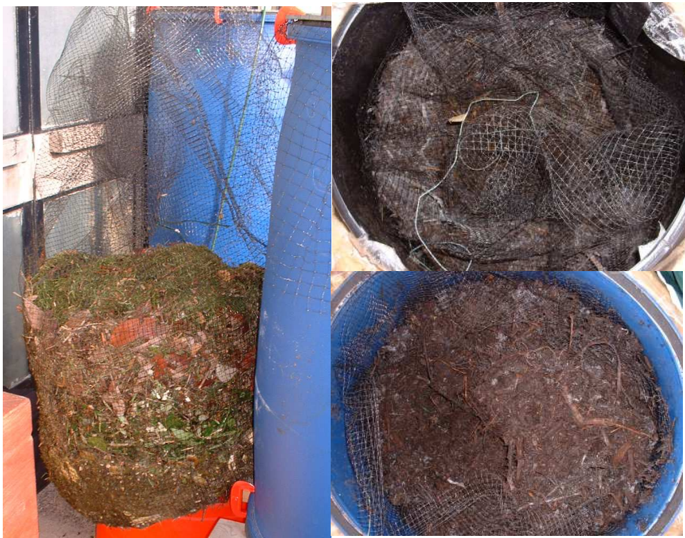
Figure 27: Use of mesh bags in composting experiments
