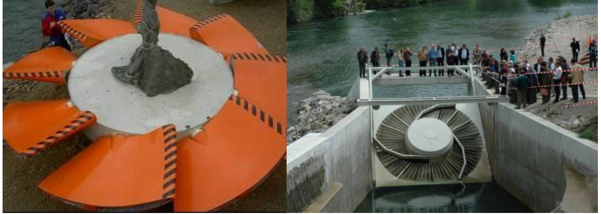
Figure 3.26: Very Low Head Turbine : a) runner b) installed (Leclerc 2009)
