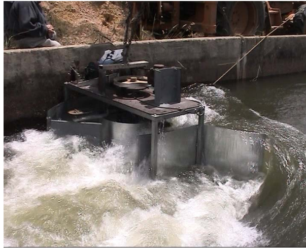
Figure 3.15: Sundermann Turbine prototype (Sundermann 2008)
