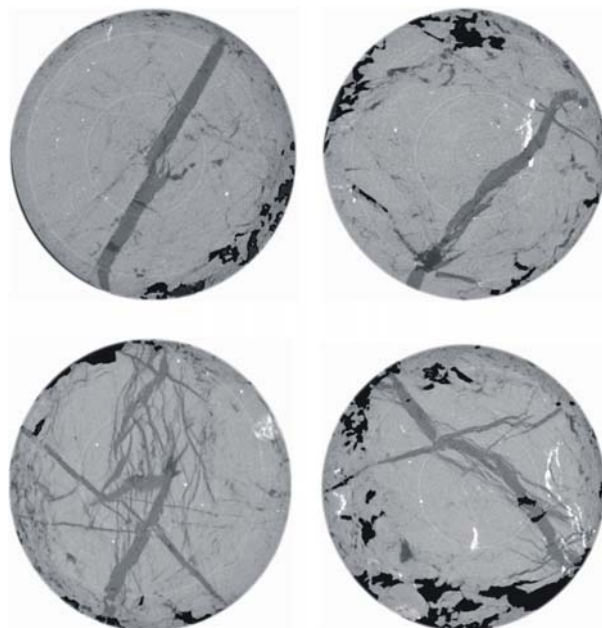
Figure 3. Horizontal slices through section core section NGHP-01-10B-08Y-6-26 cm using the X-Tek CT 160Xi.
