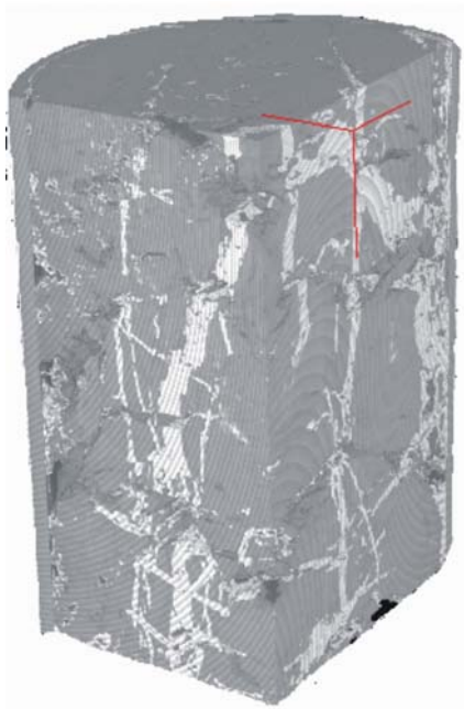
Figure 7. 3-D X-ray CT scan for the bottom of core section NGHP-01-10B-08Y-6-26 cm.
