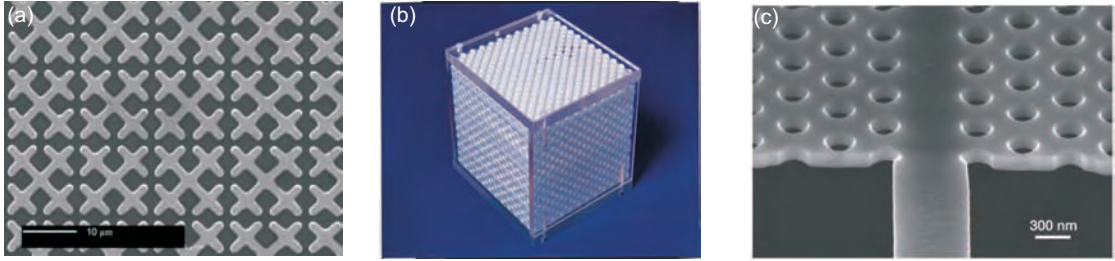
Fig. 1.4: (a) Mid-infrared multi-band FSS [25]. (b) Three-dimensional photonic crystal [26]. (c) Photonic crystal waveguide that exhibits slow light behaviour [27].
