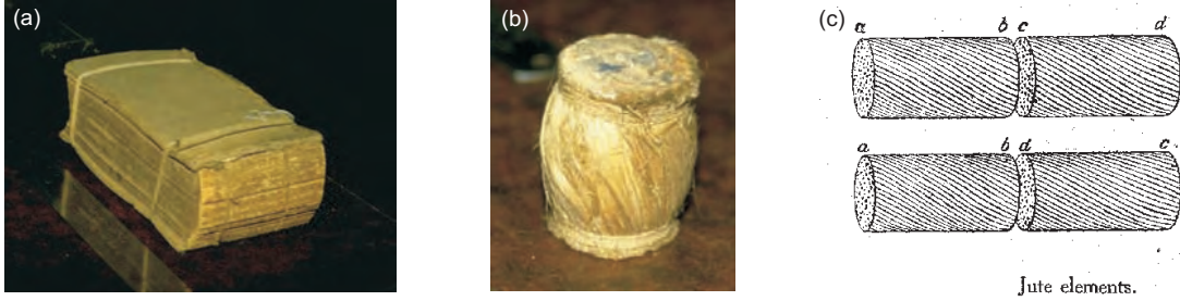
Fig. 1.3: (A stack of aluminium plates placed between the pages of a railway catalog (a) and a twisted jute ensemble (b)-(c) employed by J. C. Bose in polarization experiments with mm-wave radiation [12].
