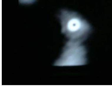
Fig. 2. Near field output of the ASE radiation guided by the silicon filled optical fibre
