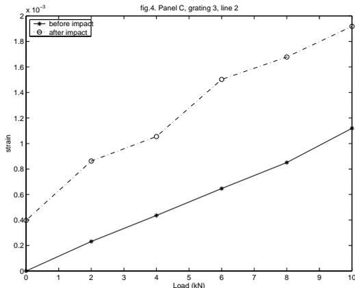
The damage observed was consistent with the differing properties afforded by the two types of test specimen. Whilst the addition of the aluminium layer greatly increased the strength of the material particularly in the transverse direction the increase in ductility which this configuration offered resulted in more energy absorption and hence damage.
