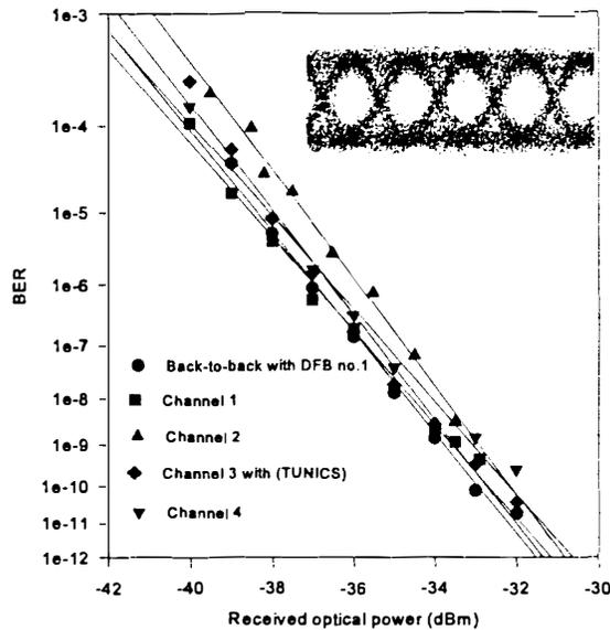
*Fig. 3. Bit-error-rate (BER) performance of simultaneous 4x10 Gbit/s WDM transmission system. (Insert) Dispersion compensated eye of channel 4.*
