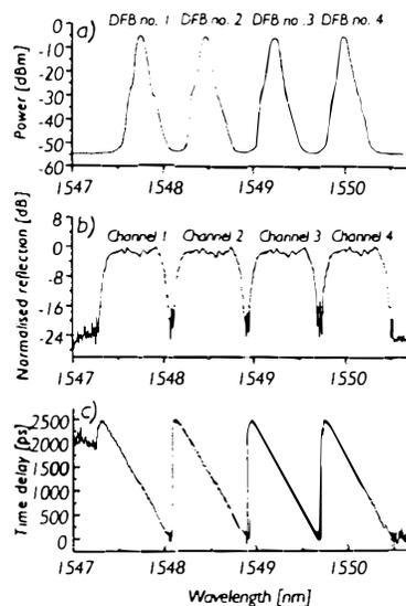
**Fig.2.** a) DFB lasing spectra after the modulator. b) Reflection and c) time delay characteristic of the 4 channel chirped sinc-sampled fibre Bragg grating.
