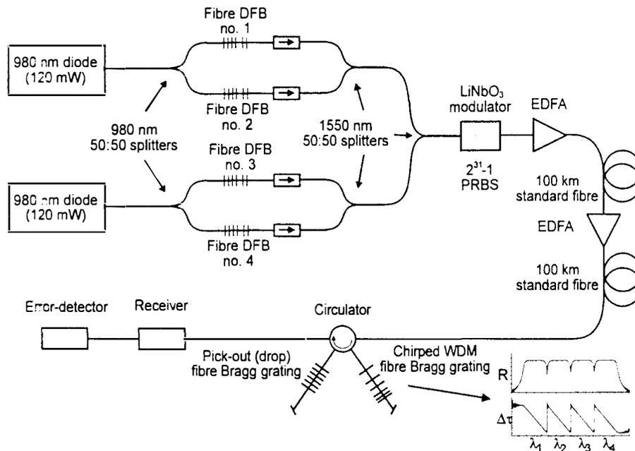
**Fig.1.** Schematic diagram of the experiment setup employing all-fibre DFB lasers as transmitter sources.
