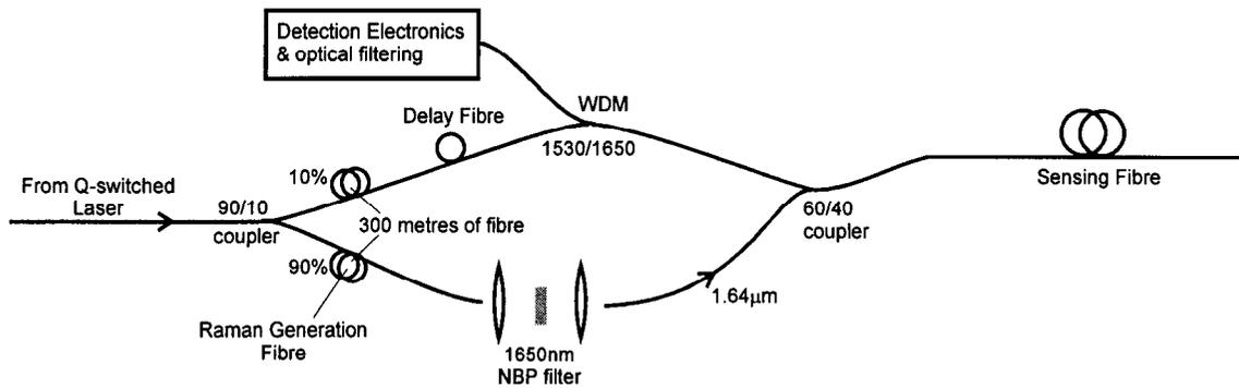
Figure 1: Set-up for Raman amplification experiment
