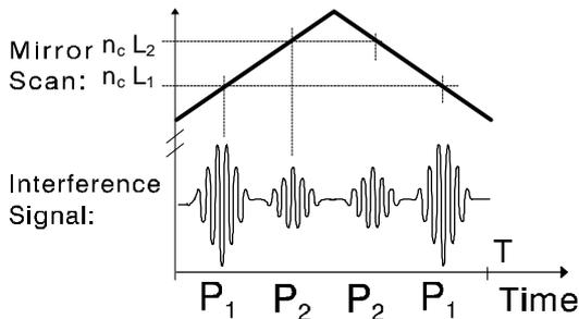
**Fig. 2 Schematic view of the interference visibility of two grating pairs  $P_1$  and  $P_2$  during scanning (in each direction) the armlength imbalance in the readout interferometer through their spacings,  $L_1$  and  $L_2$  ( $n_c$  - effective refractive index of fiber core).**
