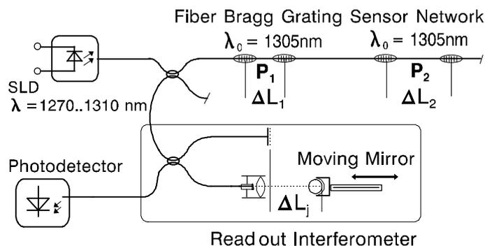
**Fig. 1 Evaluation scheme of our new coherence domain multiplexed fiber grating sensor based on pairs of Bragg gratings and scanning readout interferometer.**
