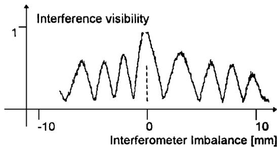
**Fig. 3 Interference visibility of a single Bragg grating reflection, as a function of readout interferometer armlength imbalance.**
